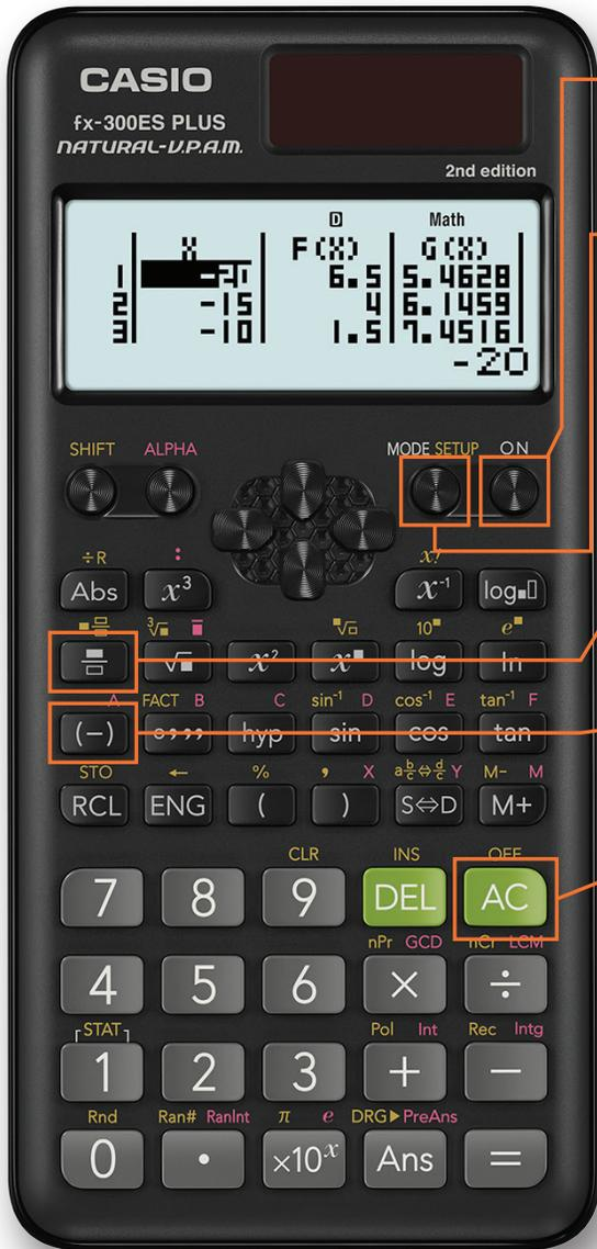
Use the **ON** key to turn the calculator on, and press **SHIFT AC** (OFF) to power the unit down.
